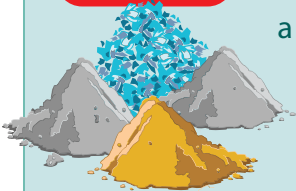
Ingredients of Glass: sand, limestone, soda ash and cullet
